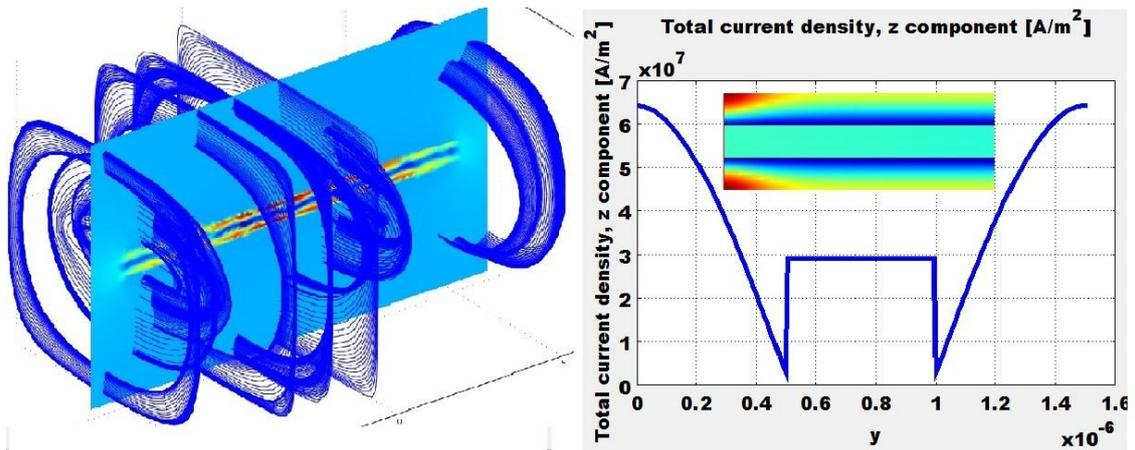
Fig. 1. (A) Outside circumferential magnetic flux density and (B) cross-section current density of FeNi/Cu/FeNi multilayer under external magnetic field of 5 Oe.
