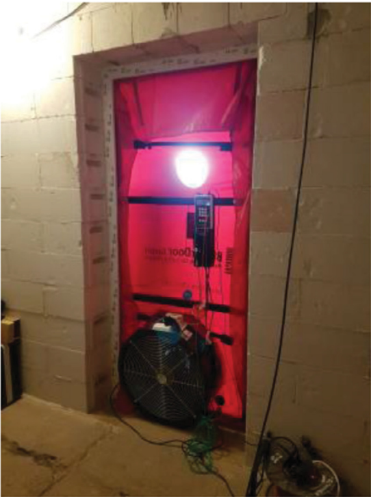
Figure 4: Blower door equipment.
