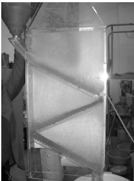
Figure 2. Counterflow coolers with louvers. The movement of the material in the laboratory model.
