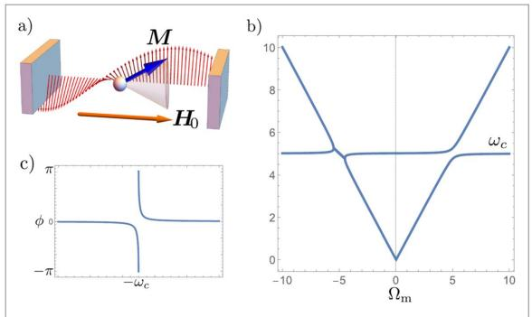
Figure 1. (a) Schematic picture of a small ferromagnetic sample interacting with circularly polarized electromagnetic wave inside a microwave cavity. (b) Energy dispersion for the Hamiltonian (1) as a function of  $\Omega_{\rm m}$  showing level repulsion near  $\omega_c$  and level attraction at  $-\omega_c$ . (c) Phase shift in the equation (2) as a function of  $\omega$  demonstrating  $2\pi$  jump near  $-\omega_c$ .
