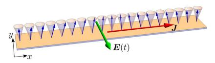
**Figure 3.** Schematic picture of a spin wave inside a small ferromagnetic specimen carrying spin current J along the x direction interacting with the cavity electric field E polarized along the y axis. The electric field is supposed to be homogeneous on the specimen's length scale.
