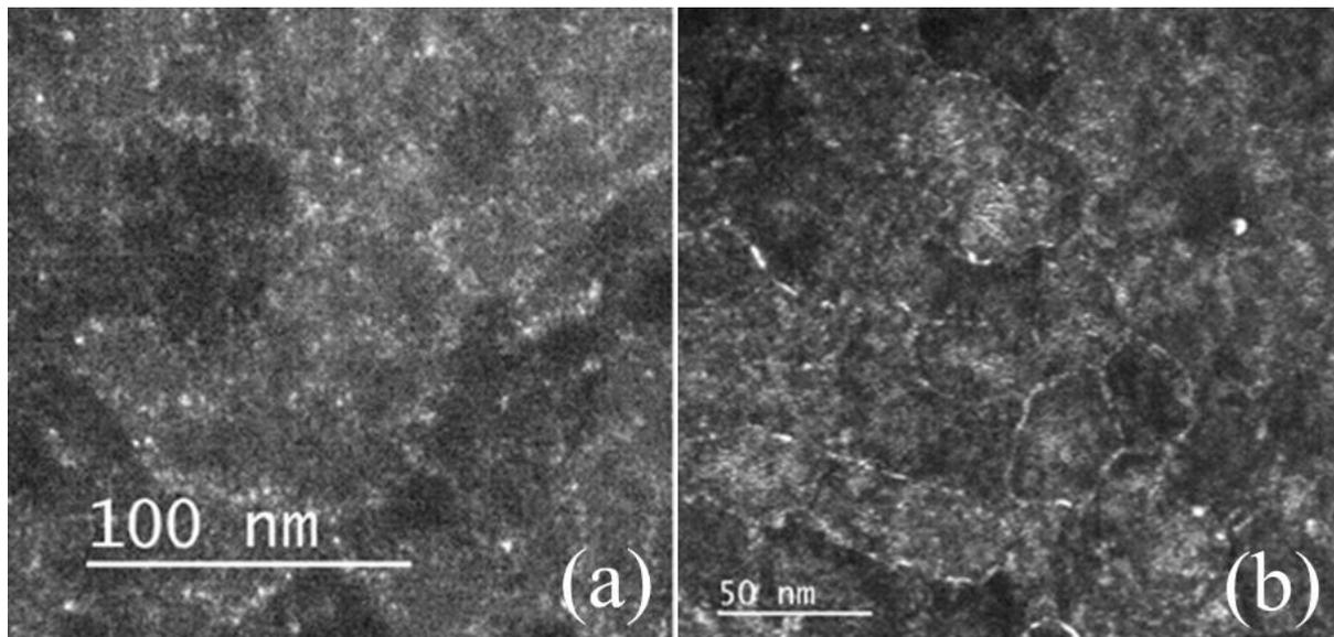
**Figure 8.** Dark-field images in (1-10) reflection of a cross section TEM image of the multilayers  $\text{Co}_{90}\text{Fe}_{10}/\text{Cu}$  (a) and  $\text{Co}_{65}\text{Fe}_{26}\text{Ni}_9/\text{Cu}$  (b).
