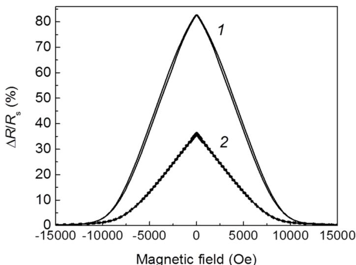
**Figure 1.** Field dependencies of the magnetoresistance of  $\text{Ta}(5)/\text{NiFeCr}(5)/[\text{FM}(1.5)/\text{Cu}(0.95)]_{32}/\text{Ta}(5)$  multilayers with FM: (1) –  $\text{Co}_{90}\text{Fe}_{10}$  and (2) –  $\text{Co}_{65}\text{Fe}_{26}\text{Ni}_9$ .
