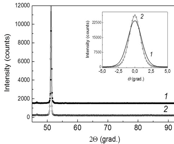
**Figure 3.** XRD patterns obtained for the (1)  $\text{Co}_{90}\text{Fe}_{10}/\text{Cu}$  and (2)  $\text{Co}_{65}\text{Fe}_{26}\text{Ni}_9/\text{Cu}$  multilayers. The inset shows the corresponding rocking curves.
