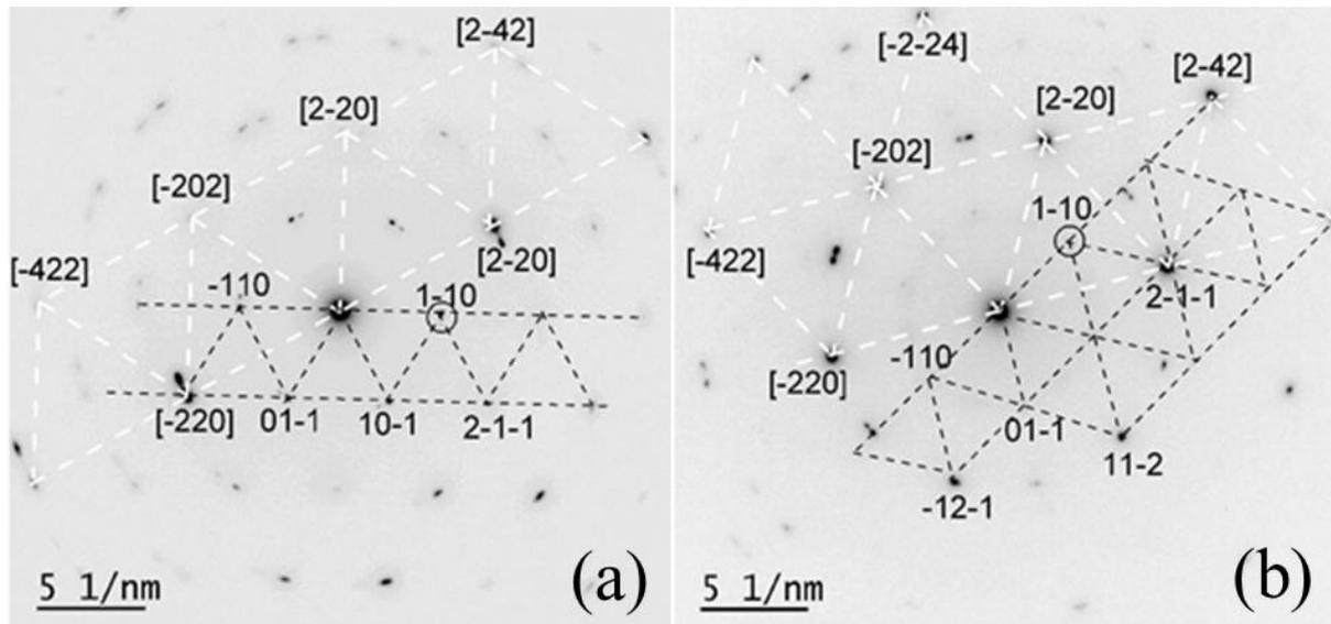
**Figure 7.** Electron diffraction patterns of the multilayers  $\text{Co}_{90}\text{Fe}_{10}/\text{Cu}$  (a) and  $\text{Co}_{65}\text{Fe}_{26}\text{Ni}_9/\text{Cu}$  (b). White and black dash lines refer to fcc and bcc network of triangles. Square frames indicate the fcc reflections.
