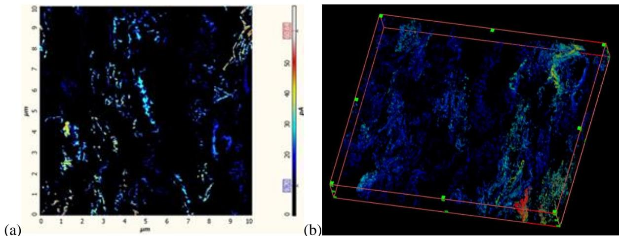
Figure 1. Current distribution images of PS-Gr composite: (a) conductive-AFM image; (b) volume 15.7x13.6x1.4 micrometers, z-step 180 nm, 9 slices.
