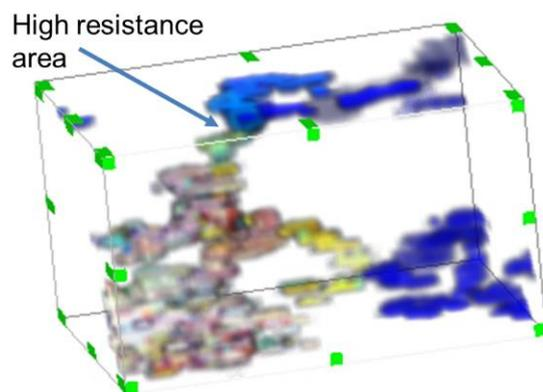
Figure 2. Epoxy-CB composite. The arrow indicates area with high resistance, which determines conductivity of neighboring domain. 28 scans, z-step is 20 nm.
