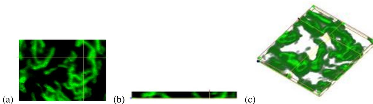
Figure 3. 3D reconstruction of PS-Gr composite by using EFM: (a) EFM image, (b), (c) cross-section and 3D reconstruction of volume structure based on 8 slices.
