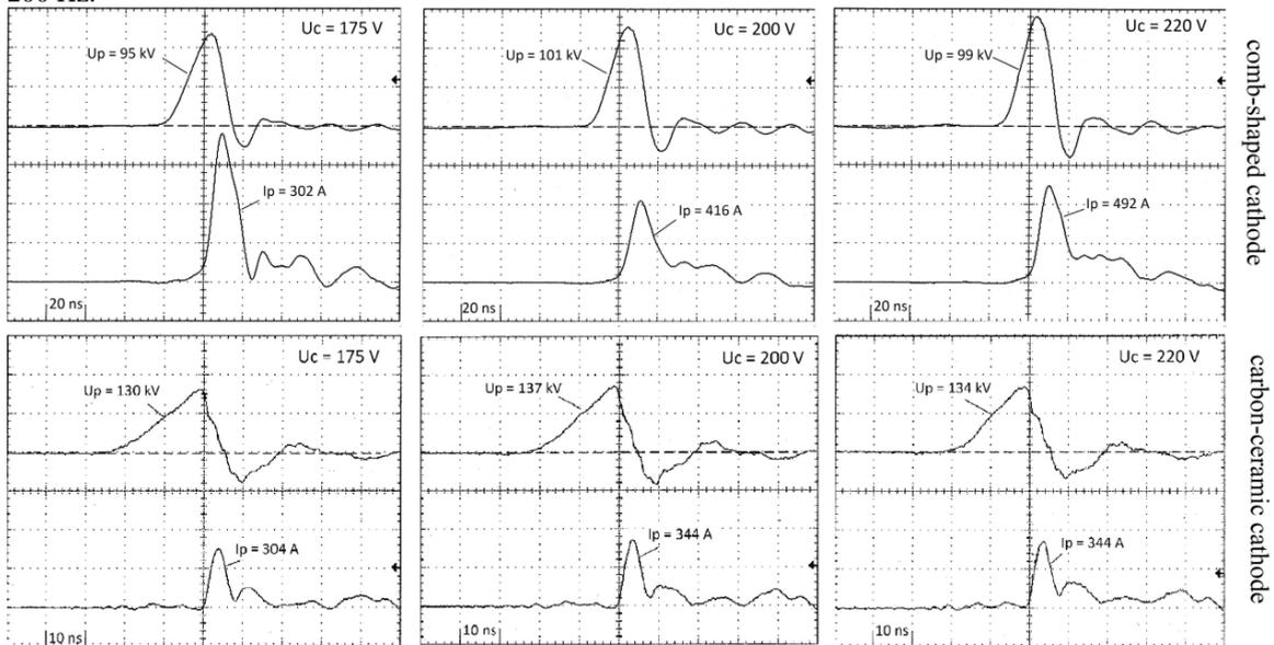
Figure 5. Waveforms of current and voltage pulses
