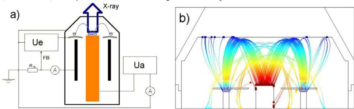
Figure 2. X-ray tube with field emission cathode
