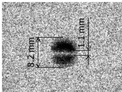
Figure 3. X-ray image of resistor pin with the characteristic dimensions. Overall spot size including penumbra is 8.2 mm.
