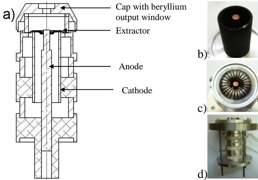
Figure 1. Model of X-ray tube with carbon field emission cathode:
