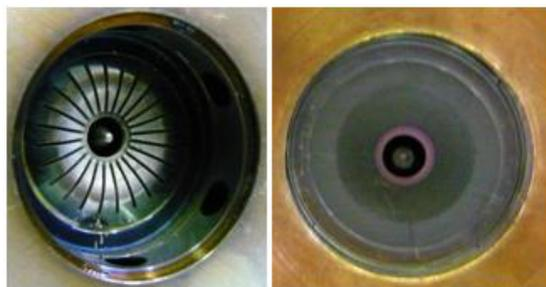
Figure 4. Photographs of X-ray irradiators with different cathodes: left – comb-shaped, right – carbon-ceramic
