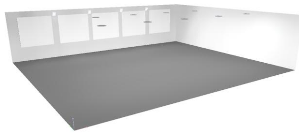
Figure 3. 3D-visualization of the swimming pool illuminated by 4 halogen floodlights TDM IO1000 SQ0301-0005 and 9 HLGs LEDsolarspot® 900. The calculation has been carried out in the augmented DIALux program
