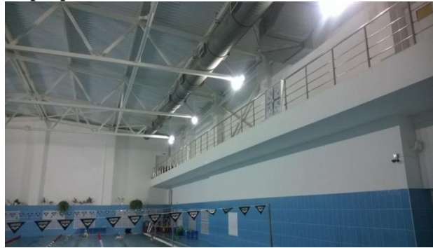
Figure 1. Photograph of the of the swimming pool interior where it is proposed to use energy efficient lighting systems based on hollow tubular light guides with a diameter of 900 mm of Solarspot International SRL company instead of halogen floodlights
