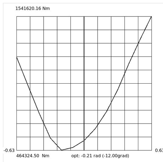
**Figure 2.** The dependence of the moment on the difference in the angles of rotation of the cranks of the crane drive and the balancing weight
