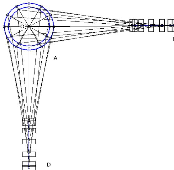
**Figure 1.** Kinematic chain of the main drive of the cold rolling mill
