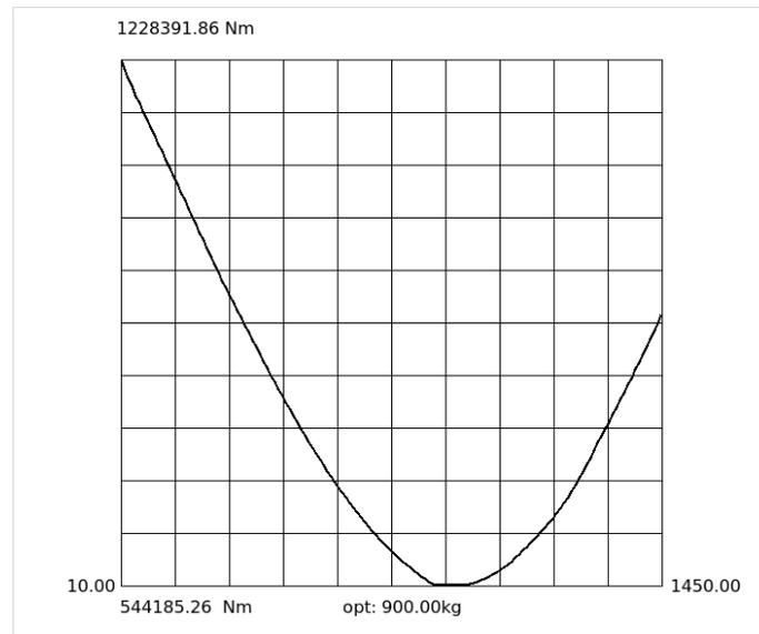
**Figure 3.** The dependence of the moment on the mass of the balanced cargo. All the parameters of the balanced circuit are related to each other. For the values obtained, the best connecting rod length of the counterbalancing load is 1.1 meters.
