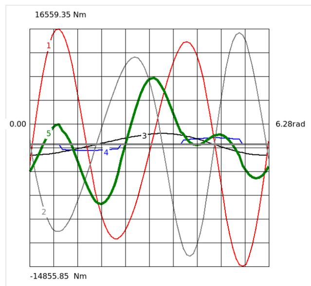
**Figure 4.** Kinematic diagram with the selected parameters and graphs of the moment dependencies on the selected parameters (1 is the moment of inertia of the second kind of stand, 2 is the moment of inertia of the second kind of the counterbalancing load, 3 is the static moment of the counterbalancing load, 4 is the technological moment, and 5 is the total moment).
