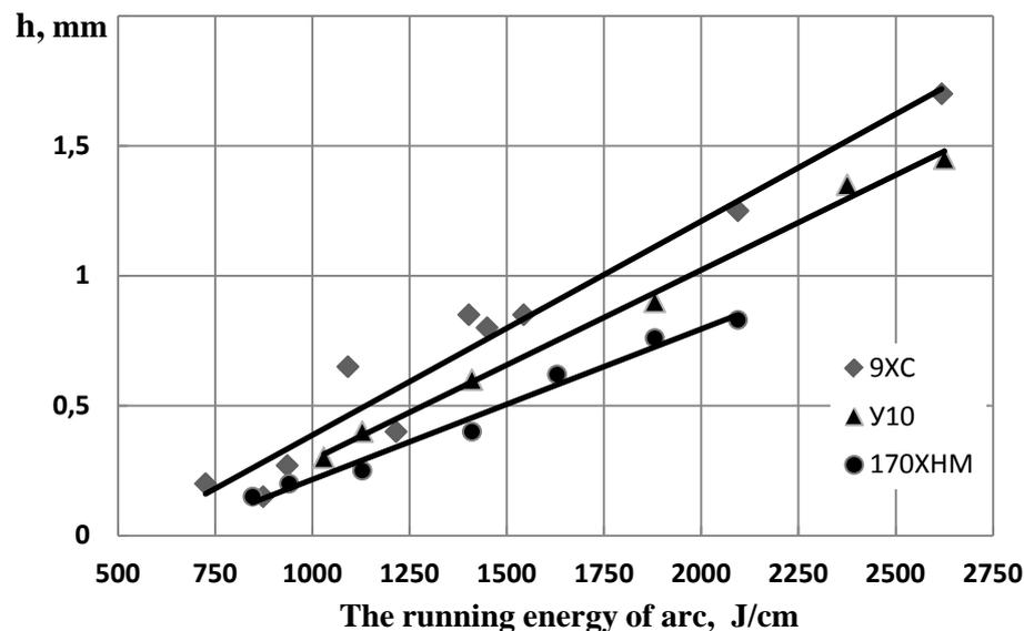
**Figure 1.** Influence of the running energy of arc on the depth (h) of the zone of plasma quenching of hypereutectoid steels.
