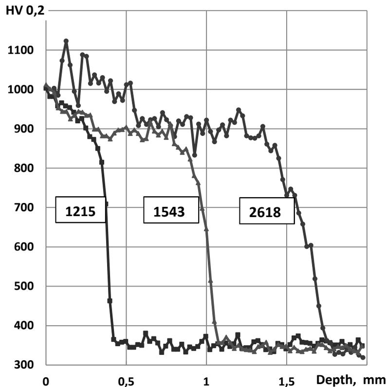
**Figure 3.** A change in the microhardness along the depth of the local zone of plasma quenching of 9XC steel at different running energy of arc values (J/cm).
