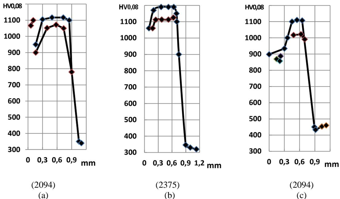
**Figure 2.** A change in the microhardness (HV 0.08) over the depth of the plasma quenching zone of steels: 9XC (a), Y10 (b), 170XHM (c) for different values of running energy of arc (J/cm).
