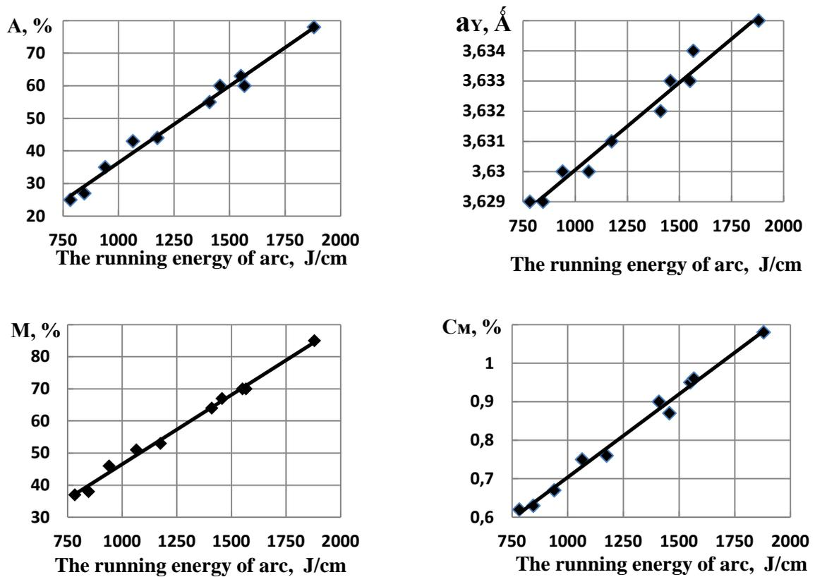
**Figure 4.** The effect of the running energy of arc in the plasma hardening of steel Y10 on the volume fraction of the residual austenite in the surface layer ( $A$ , %), the austenite lattice parameter ( $a_{\gamma}$ , Å), the volume fraction of the martensite of quenching in the composition of the  $\alpha$  phase ( $M$ , %), the carbon concentration in martensite quenching ( $C_M$ , %).
