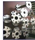
Fig.2. Photos of vortex inserts: a) with three grooves; b) with twelve grooves; c) - a set of investigated samples of vortex inserts with different internal surface geometries.
