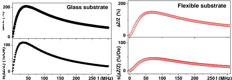
$nm)/[Ti(6 nm)/FeNi(170 nm)]_3$  multilayer deposited onto glass and flexible substrates.
