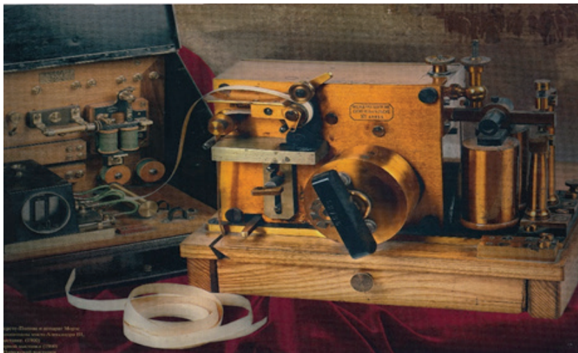
A radio receiver by A. S. Popov with a connected Morse telegraph unit
