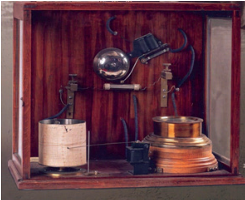
The first radio receiver by A. S. Popov (1895)
