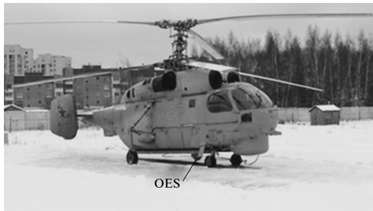
Fig. 1. An OES-based helicopter complex of radiation monitoring.
