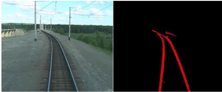
Figure 6: Results of intelligent algorithm for \sigma = 2 and threshold = 100 .
