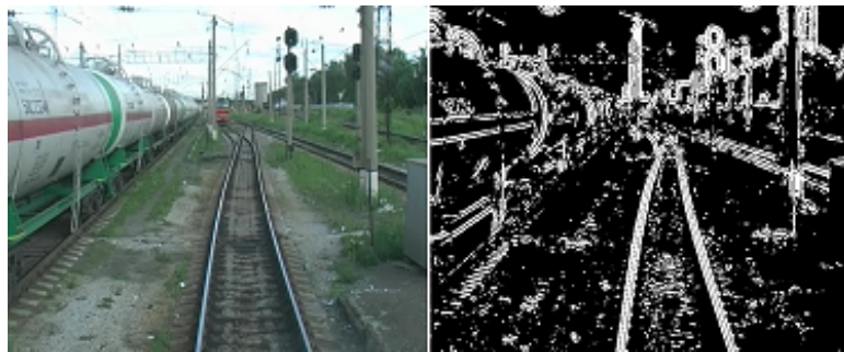
Figure 2: A threshold filter with threshold = 100.
