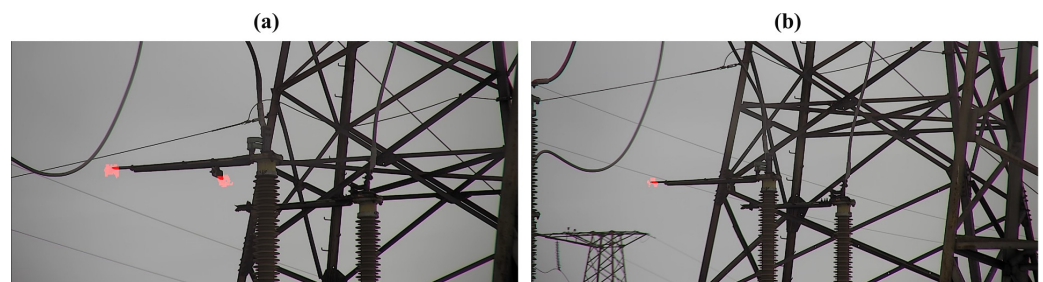
Figure 1. The example of the same corona discharge activity recorded from the distances of (a) 28 m and (b) 37 m using the Ofil Rail HD UV camera with the same UV channel gain. The images are generated by combining a frame from the RGB channel with the average corona activity registered by the UV channel during 9 s periods (red zones).
