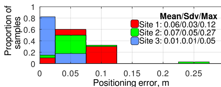
Figure 8. Histograms of positioning error recorded at different experimental sites at the inspection missions' keypoints.
