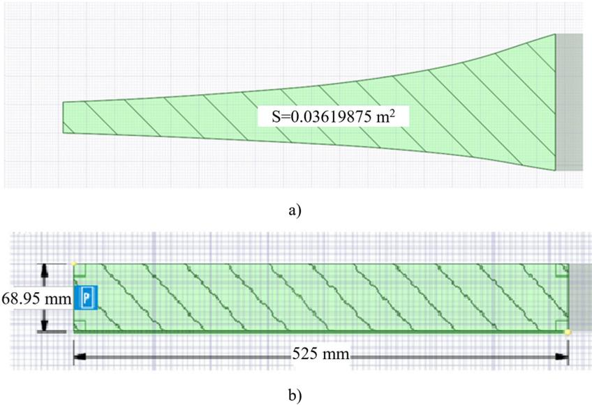
**Fig. 4.** Cross-sectional area of the swept volume of the fan blades and virtual disk: a) the cross-sectional shape formed by the rotation of the fan blades of the actual design; b) cross-sectional shape formed by the rotation of the virtual fan blades.
