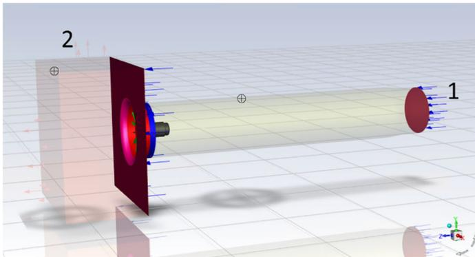
**Fig. 7.** Boundary conditions: 1 – entrance to the computational domain; 2 - exit from the calculation domain.
