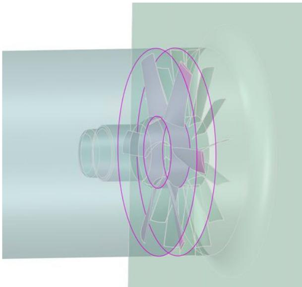
**Fig. 1.** Calculated geometry of a virtual test bench with real fan geometry.
