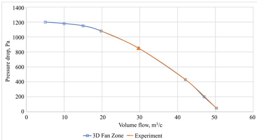
**Fig. 5.** Flow-pressure characteristics of the 3D Fan Zone fan.
