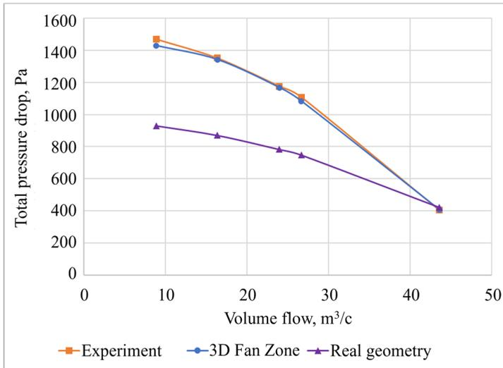
**Fig. 8.** Graph comparing the results of physical and numerical modeling of a fan as part of a test bench.
