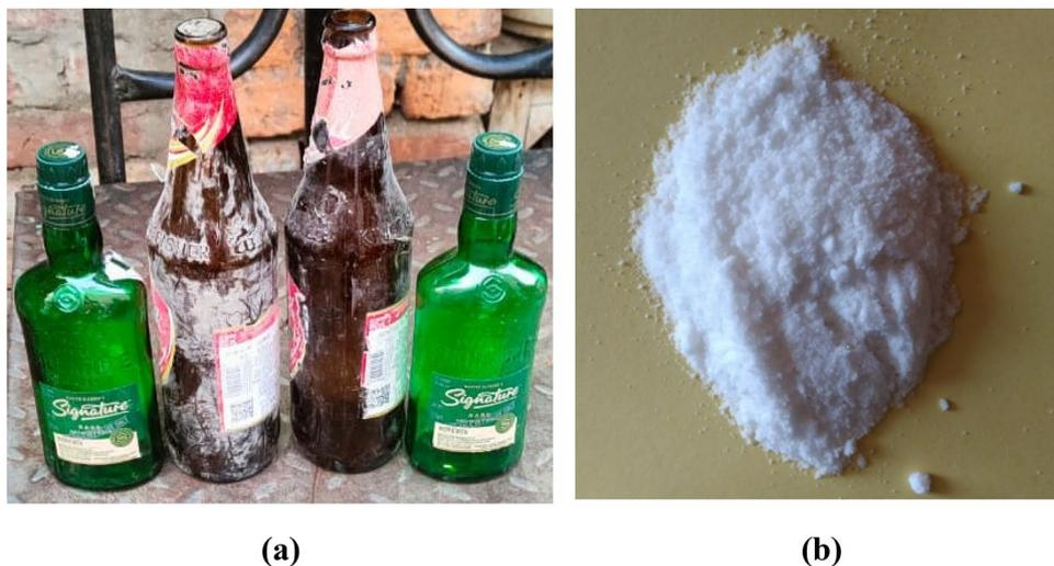
**Figure 4.** Illustration of (a) Waste-glass, (b) WGP particulates.
