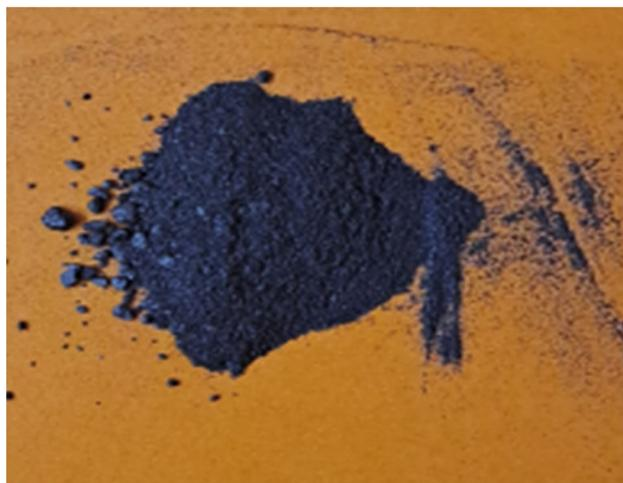
**Figure 7.** Illustration of silicon nitride ( $\text{Si}_3\text{N}_4$ ) powder.
