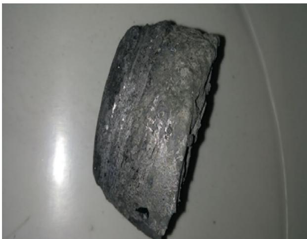
**Figure 11.** Photograph of developed Si<sub>3</sub>N<sub>4</sub>/WGP/AZ91D Mg-MMCs samples.
