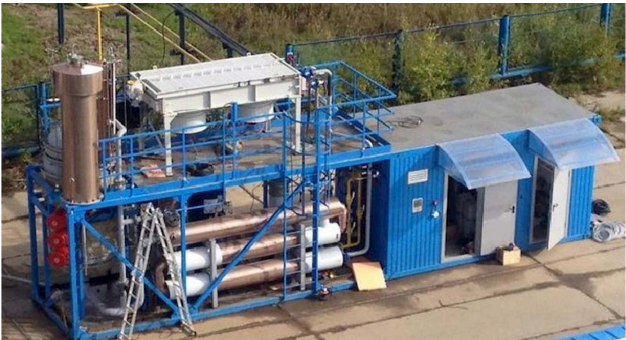
Figure 2. Full size prototype of APG conversion unit.
