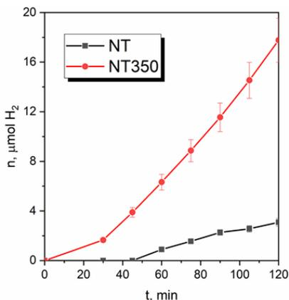
**Figure 1.** Kinetic curves of the photocatalytic hydrogen production over NT and NT 350 photocatalysts under UV-irradiation.
