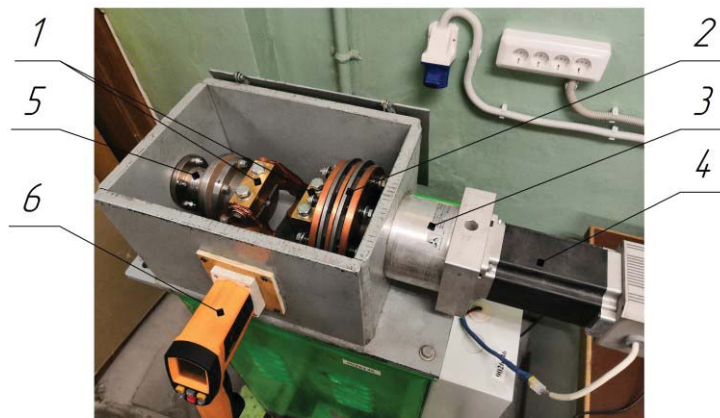
FIGURE 2. The torsion test setup: 1 – grips; 2 – sliding electric contact; 3 – planetary gearbox; 4 – step motor drive; 5 – torque sensor; 6 – pyrometer
