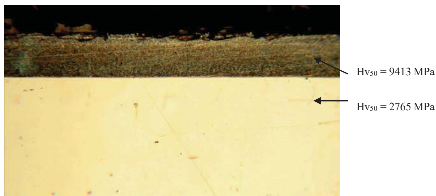
FIGURE 4. Aluminized alloy Hastelloy G35 at 800 °C. Layer thickness is 70 \mu\text{m} .
