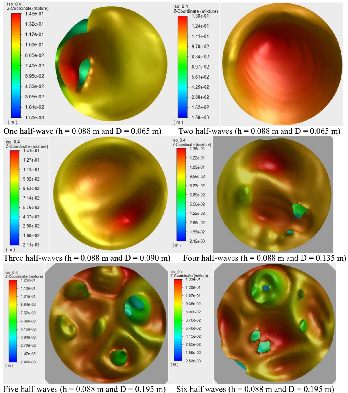
**Figure 3.** Surface of a fluidized bed at different numbers of half-waves.
