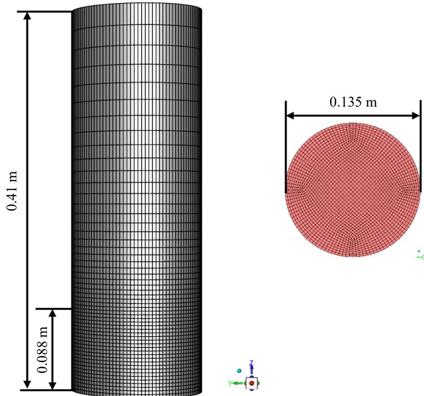
**Figure 1.** Mesh for case with  $D = 0.135$  m.
