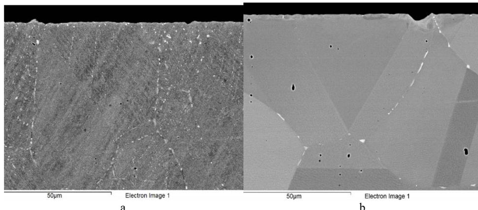
**Fig. 6.** SEM images showing the microstructure of steel 316L obtained by traditional metallurgical technology after corrosion tests. a - without preliminary heat treatment, b - after annealing at 1200 ° C, 1 h
