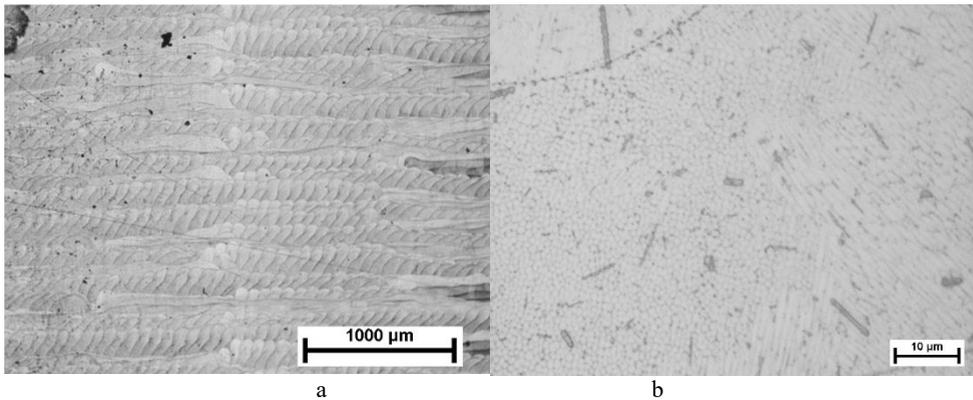
**Fig. 2.** OM images showing the sample microstructure after SLM along the growth direction.
