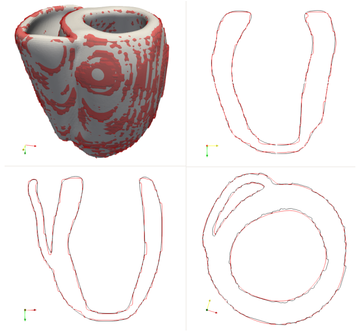
Fig. 3. Two representations of the object: SDT (red) and SDF (black or white). Note the smoothness effect of the implicit representation with MLP.
