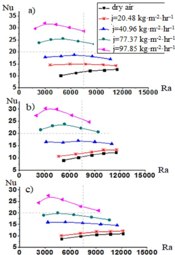
**Fig. 6.** The influence of water concentration  $j$  on the cylinders' cooling in the channel: a – the first row, b – the second row, c – the third row.
