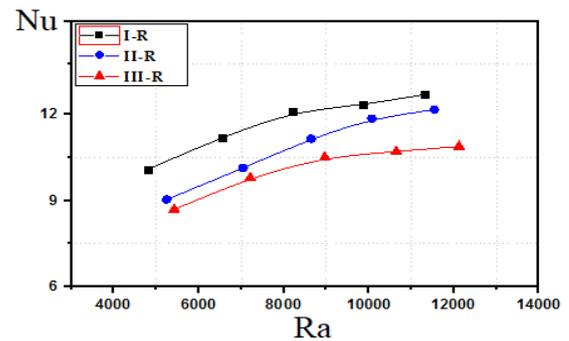
**Fig. 5.** The cooling of the cylindric elements in the channel in conditions of natural convection for the 1<sup>st</sup>, the 2<sup>nd</sup> and the 3<sup>rd</sup> rows (see Fig. 2).
