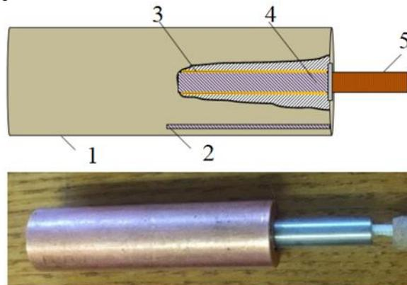
**Fig. 3.** The scheme and the photograph of a heat-exchange tube: 1 – the cylindric heating element; 2 – the thermocouple; 3 – the heat-conducting paste; 2 – the electric heater; 5 – the textolite rod.
