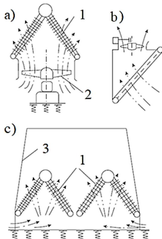
**Fig. 1.** Ways of cooling air supply: a – forced circulation with pressurization, b – forced circulation with depression, c – natural circulation; - - - - cooling air; 1 – heat-exchange surface; 2 – fan; 3 – tower.
