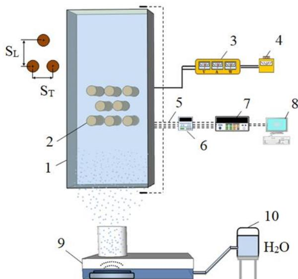
**Fig. 2.** The schematic diagram of the experimental facility: 1 – the heat-insulated channel; 2 – the tubes of the heat exchanger; 3 – the multimeter; 4 – the voltage regulator; 5 – the thermocouples; 6 – the analog output module; 7 – the data acquisition module; 8 – the computer; 9 – the ultrasonic water mist generator; 10 – the water tank.
