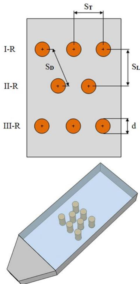
**Fig. 4.** The arrangement of tubes in the channel.
