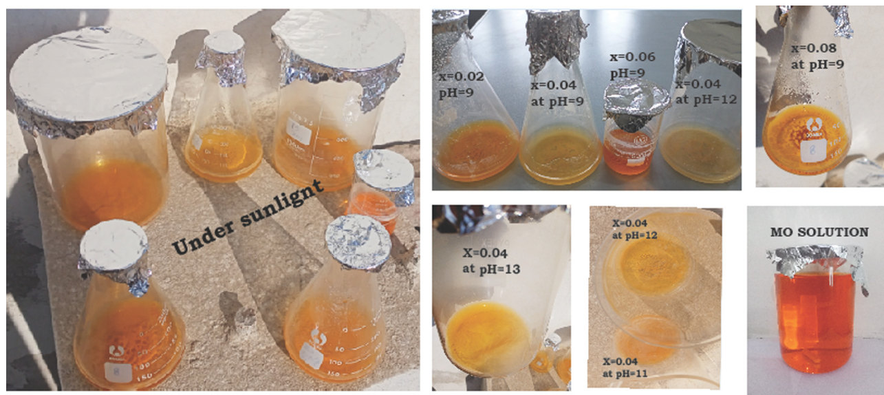
Fig. 8. Photocatalytic degradation of samples under sunlight.
