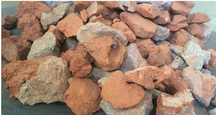
Figure 1. Appearance of crushed scrap of wall structures.
