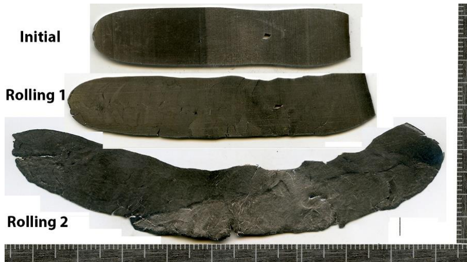
Figure 1. EBM rhenium workpiece under the cold rolling: (i) initial state; (ii) rolling on 18%; (iii) rolling on 45% (after annealing 30mnutes at 1400°C).
