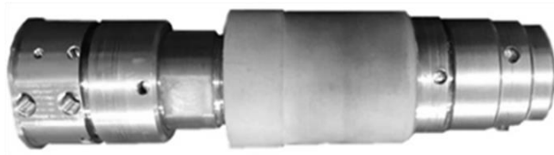
Figure 6. Pilot model of the plasma torch PMVR-5.3 for precision cutting of small and medium thickness metals.
