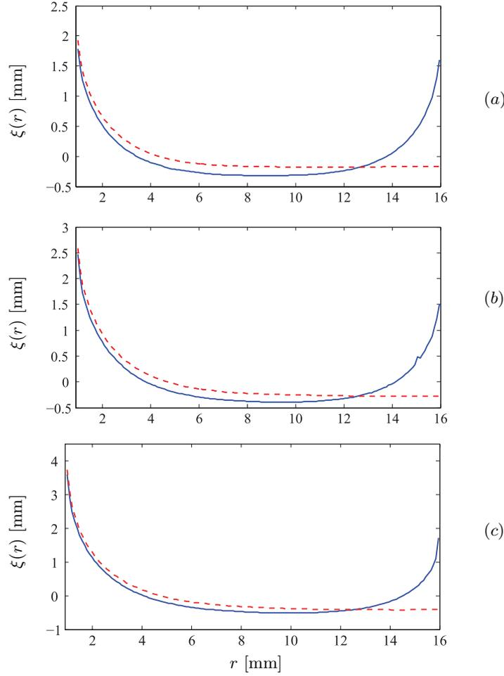
*Fig. 5.* (color online) The surface  $\xi(r)$  (blue solid line) versus the distance  $r$  from the wire as a function of current with the condition  $\phi_1 = \phi_2$ : (a)  $I = 20$  A and  $\phi_1 = \phi_2 = 8.7^\circ$ , (b)  $I = 45$  A and  $\phi_1 = \phi_2 = 6.3^\circ$ , and (c)  $I = 70$  A and  $\phi_1 = \phi_2 = 3.4^\circ$ . The red dashed line presents the surface for  $\phi_2 = 90^\circ$  for comparison. The remaining parameters are those of Fig. 3.
