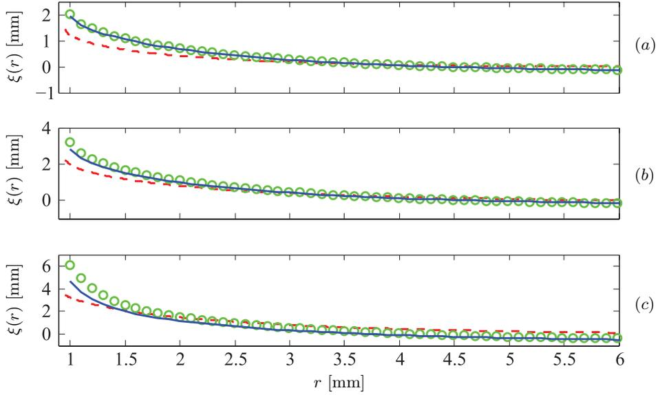
*Fig. 6.* (color online) The surface  $\xi(r)$  versus the distance  $r$  from the wire as a function of the strength of the current: (a)  $I = 20$  A ( $H \simeq 3.4$  kA/m), (b)  $I = 45$  A ( $H \simeq 7.5$  kA/m), (c)  $I = 70$  A ( $H \simeq 11.7$  kA/m). The red dashed line shows the measured profiles, the blue solid line (green circles) the calculated ones for a linear magnetization with  $\chi = 0.61$  ( $\chi = 0.8$ ). For details see the text.
