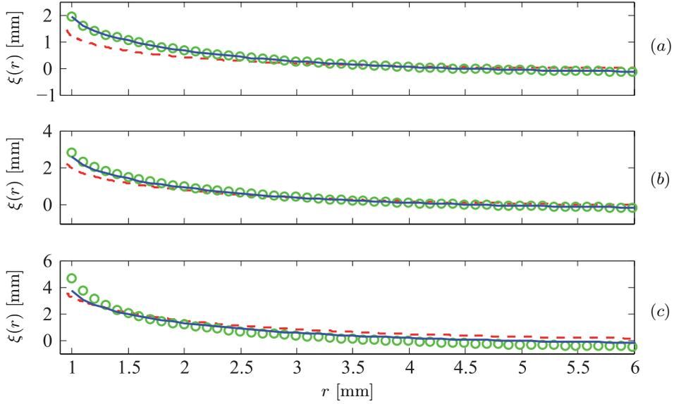
Fig. 7. (color online) The surface  $\xi(r)$  versus the distance  $r$  from the wire as a function of the strength of the current: (a)  $I = 20$  A ( $H \simeq 3.4$  kA/m), (b)  $I = 45$  A ( $H \simeq 7.5$  kA/m), (c)  $I = 70$  A ( $H \simeq 11.7$  kA/m). The red dashed line shows the measured profiles, the blue solid line (green circles) shows the calculated ones for a nonlinear magnetization (a linear magnetization with  $\chi = 0.61$ ). For details see the text.
