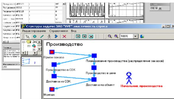
**Fig. 2.** A fragment of the industrial process model which is worked out for the “Urals Industrial Group” enterprise and made with the help of the simulation system “BPsim”. For every graph node in the form view there is an operation or RCP, for every connection between the nodes there is a resources flow, for every agent there is a model of the director of operations.
