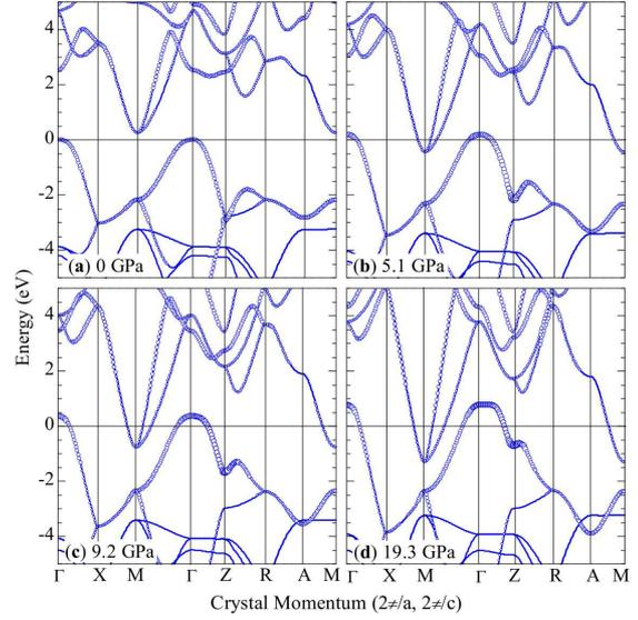
Fig. 3. Band structure plots of SnO at ambient, 5.1 GPa, 9.2 GPa, and 19.3 GPa calculated with the PBE + mBJ exchange-correlation functional. The Sn *5s* contribution to the band structure is proportional to the width of the line.
