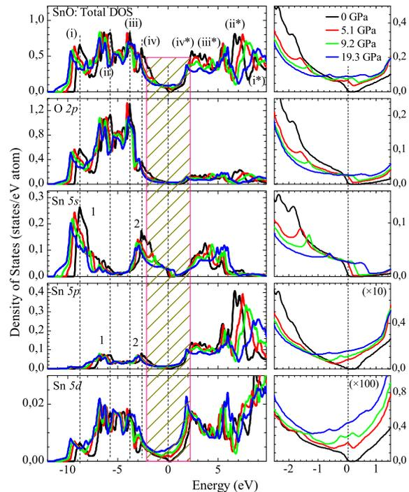
Fig. 1. Total and partial densities of states of SnO for ambient pressure and pressures 5.1, 9.2, and 19.3 GPa. The key bonding (i - iv) and anti-bonding ( $iv^*$  -  $i^*$ ) features are labeled and discussed in the text. The PBE + mBJ calculation is shown here, apart from the band gap the other calculations give very similar DOS spectra.
