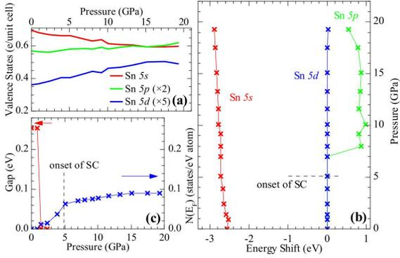
Fig. 4. The number of valence states of Sn (a), the correlation shift between the Sn and O  $2p$  states (b), and the band gap and number of states at the Fermi level (c).
