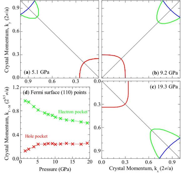
Fig. 5. One quadrant of the Fermi surface in the  $k_x$ ,  $k_y$  plane (at  $k_z = 0$ ) for SnO at 5.1 GPa (a), 9.2 GPa (b), and 19.3 GPa (c), calculated with the PBE + mBJ functional. Since our calculation suggests SnO at ambient pressures is an insulator, the Fermi surface in this case is trivial. In panel d, the nesting vector in the (110) direction from the corner of the  $\Gamma$  point hole band to the opposite outer  $M$  point electron band is also shown for various pressures.
