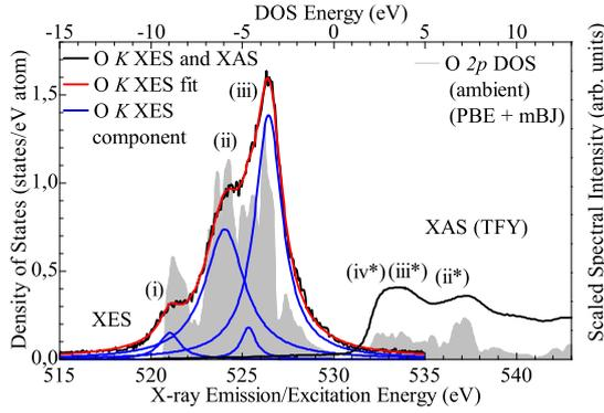
Fig. 2. The measured O *K*-edge XES and XAS. The XES spectrum has been fit with 4 pseudo-Voigt components, three of which agree with the previously discussed valence band intervals. The ambient O *2p* DOS is also plotted, it has been aligned with the XES spectrum. The XAS spectrum shows the same two intervals as the calculated DOS.
