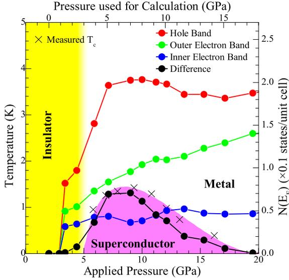
Fig. 6. Number of states at the Fermi level of the bands forming electron and hole pockets and their difference (hole band) – (inner and outer electron bands) vs. pressure. For comparison the phase diagram and pressure dependence of superconducting transition temperature from [1] are given accounting for the underestimated by 1.5 GPa energy gap closure in the calculation.
