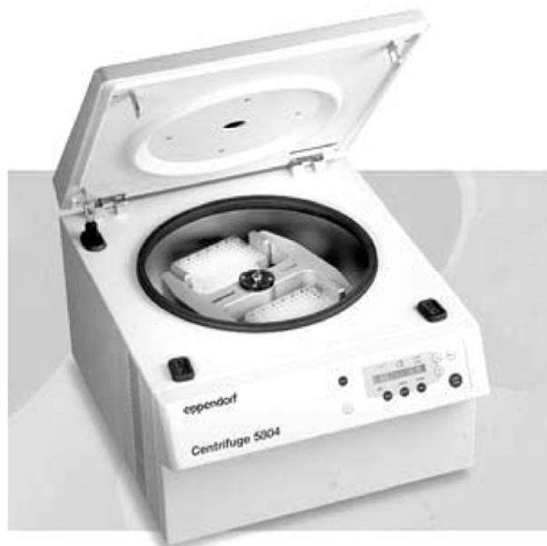
Fig. 2. Centrifuge with a rotor for microplates.
