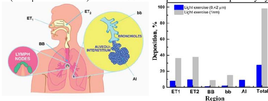
Fig. 1. Deposition fractions of attached (0.42 μm) and unattached (1 nm) radon progeny in different regions of human respiratory tract for physical exertion light exercise.
