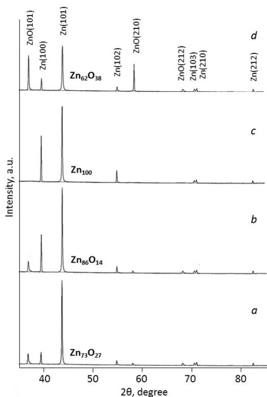
Fig. 2. X-ray diffraction patterns of Zn-based nanotubes:
