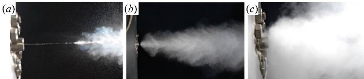
Fig. 3. Types of water jets at the expiration of the saturation line: a ) T_{0s} = 170 °C; b ) T_{0s} = 182 °C; c ) T_{0s} = 300 °C.
