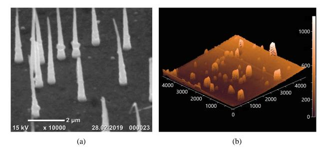
Figure 1. (a) SEM and (b) SPM-image of conical nanowires.
