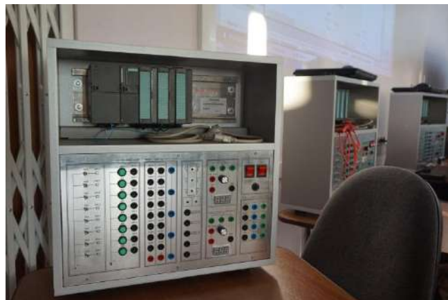
Рис. 1. S7-300 PLC-based workbench
