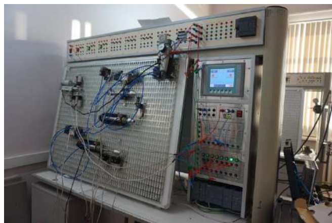
Рис. 2. S7-1200 PLC-based workbench
