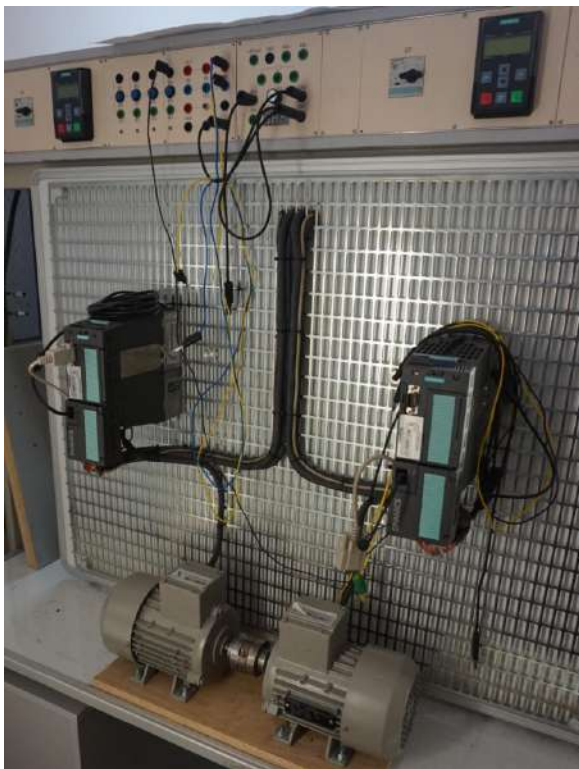
Рис. 3. A workbench based on electric drives by Sinamics
