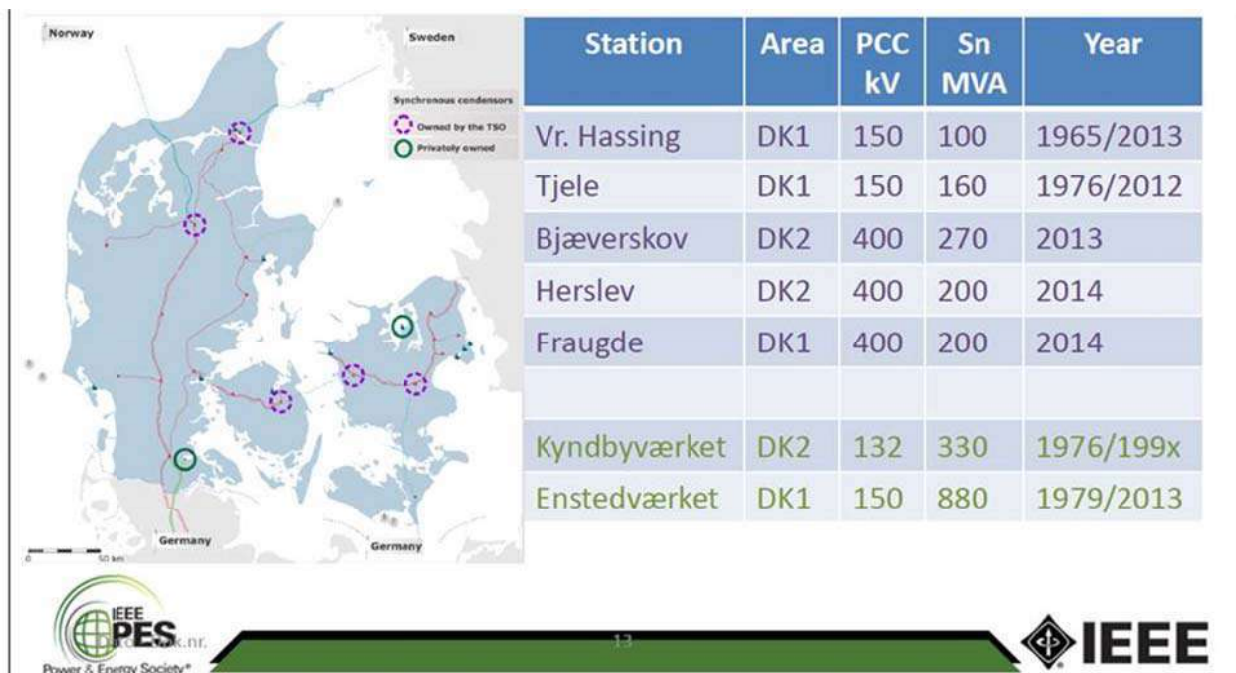
Fig. 2. Application of 2-nd generation of synchronous condenser in Denmark.
